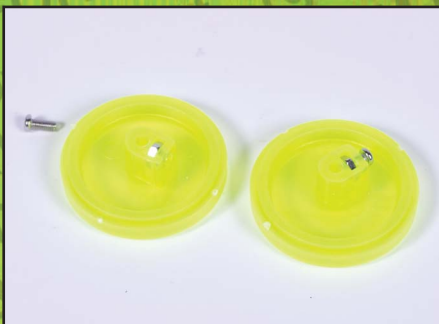
FIGURE 11. Attach two axle set screws to the main drive wheels.
